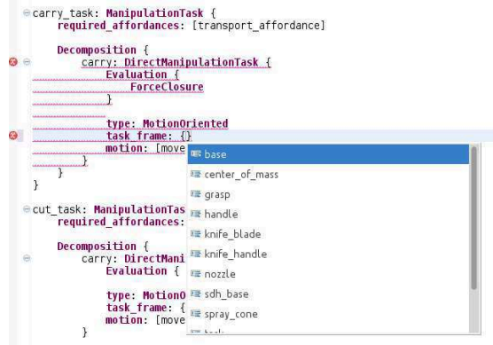
Figure 7.1.: Excerpt of the generated IDE which shows the auto-completion for GDDL
